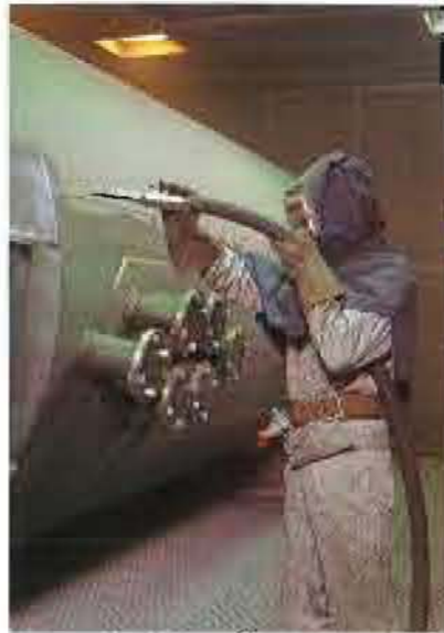
This method by spraying and built-up contains chop fibre, glass and hardener, of which is stronger when is set.
