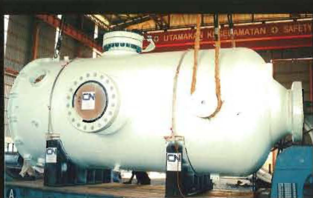
Compressor Suction Scrubber 2700 I/D x 7000 ht x 102 = 3 Thk S/S 316L Cladded
